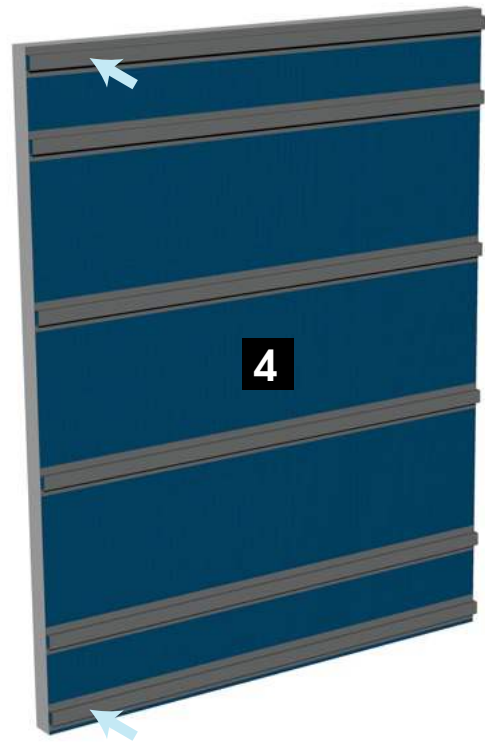
4 Install auxiliary tophats for flashings support on top and bottom of wall.
