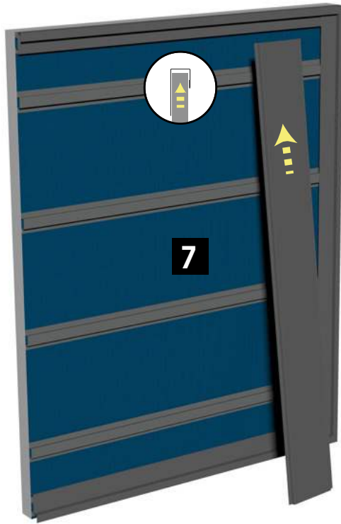
7 Slide up the first Expression™ panel into the top flashing.
