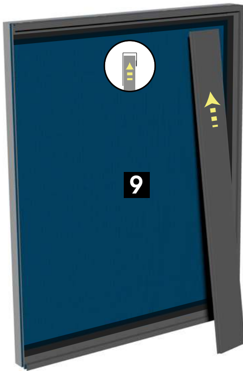
9 Slide up the first Expression™ panel into Top Flashing.
