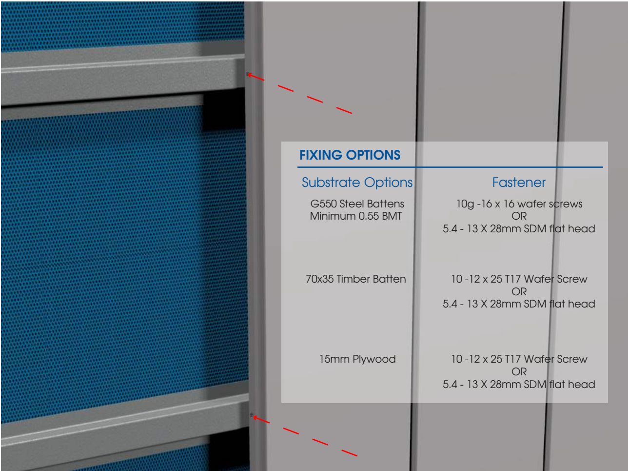
Diagram showing screw engagement on vertical Expression™ panels over steel battens. Timber battens and plywood can also be used as substrates
