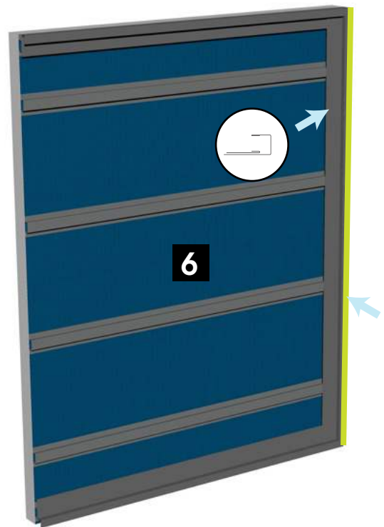
6 Install Side Wall Flashing, and then install Starter Strip. Seal Side Wall Flashing against the wall.
