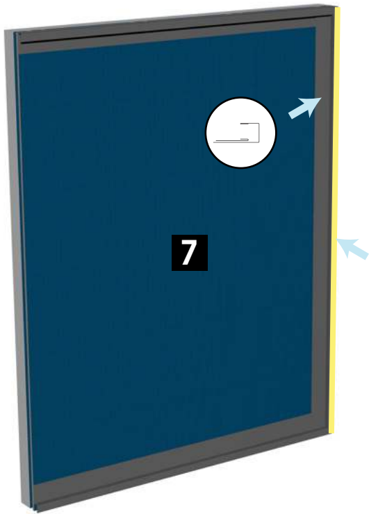
7 Install Side Wall Flashing, and then install Starter Strip. Seal Side Wall Flashing against the wall.
