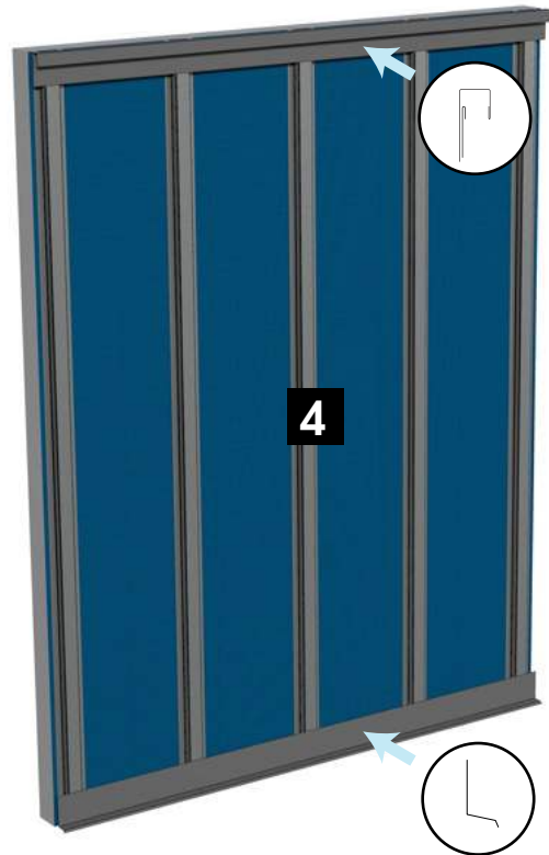
4 Install toe mould flashing at bottom and custom top flashing with a starter strip at top.
