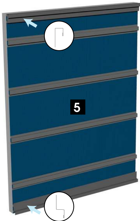
5 Install Top Flashing and Toe Mould Flashing.
